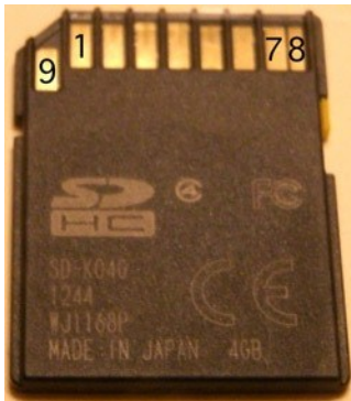
Figure 10-1. SD card pinout
